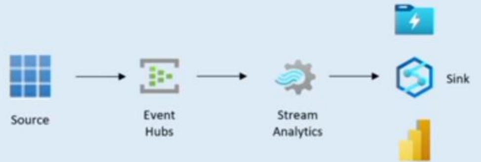
ELT Streaming Ingestion Pattern – Stream Analytics
